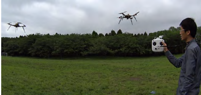
Fig. 3. Flight formation testing using 2 UAVs.
